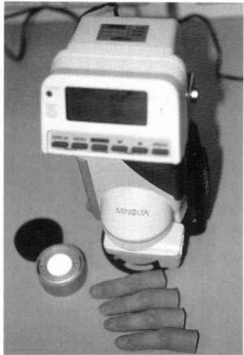
Fig 1. The spectrophotometric unit used for assessing the colour match results and the four prostheses which were prepared under illuminant TL84, F, D65 and a combination of TL84-F-D65.
