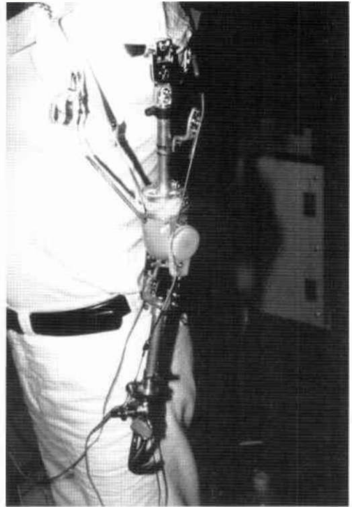
Fig. 7. Dynamic pulling test by a subject. Pulling force, hook opening force and hook opening angle are measured while the cable is pulled by a subject.
