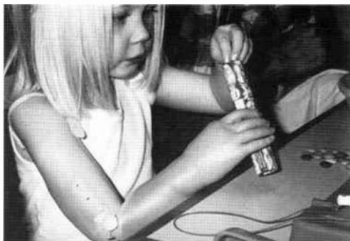
Fig 2 SCAMP myoelectric hand in use by a child with through elbow deficiency.
