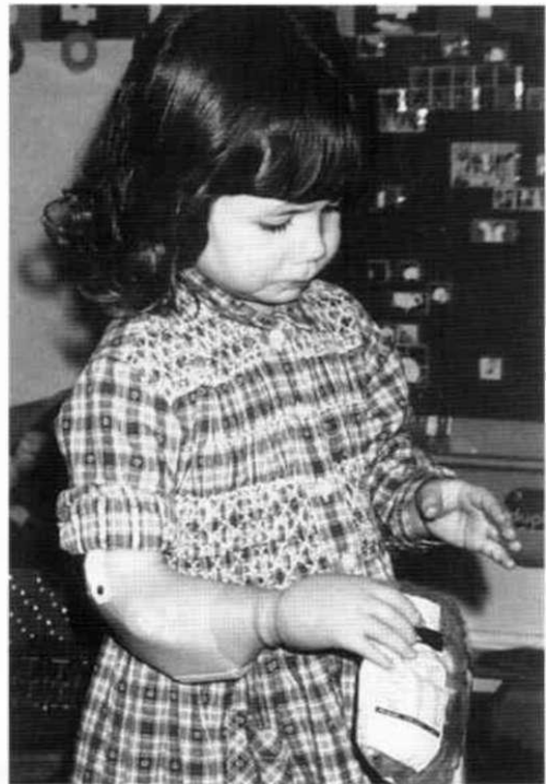
Fig. 1. SCAMP myoelectric hand in use by a child with below elbow deficiency.
