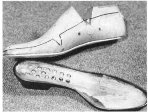
Fig. 2. The first part of the PVC shell is formed by moulding over the bottom of the last: an example sole unit is also shown.
