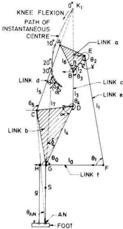
Fig. 2. Six-bar linkage knee-ankle mechanism used in the new prosthesis.
