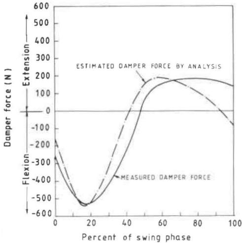
Fig. 12. Variations of forces in pneumatic damper during swing phase of walking obtained from dynamic analysis of prosthesis and experimental measurements.
