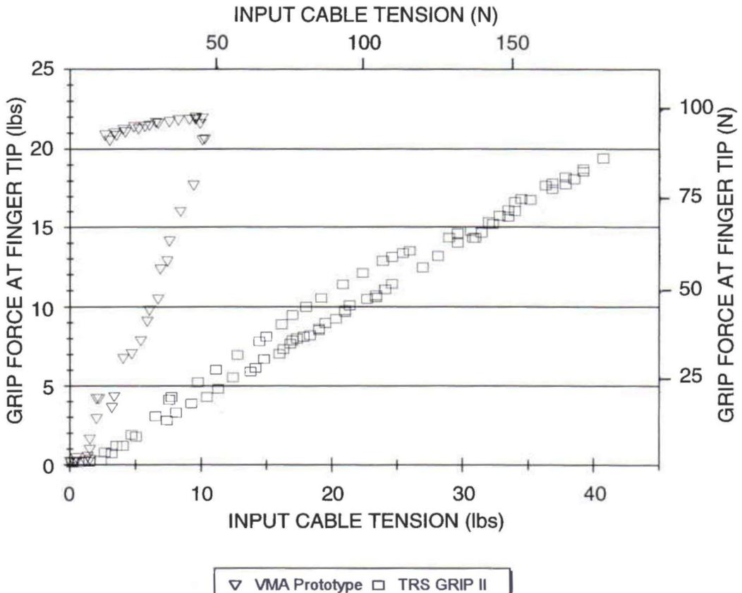
Fig. 5. The gripping performance of the VMA prehensor compared to that of a conventional voluntary closing device (the TRS GRIP II).
