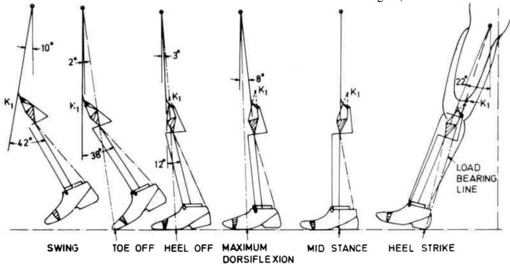
Fig. 8. Positions of instantaneous knee centre of the prosthesis with reference to the line passing through hip joint and centre of contact of foot with ground at different phases of walking
