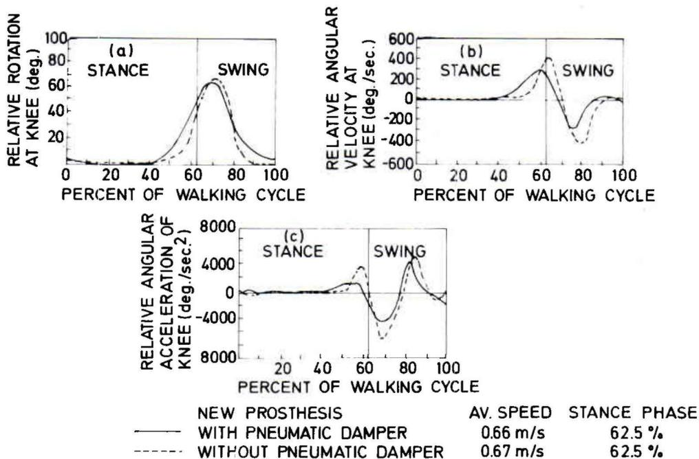
Fig. 11. Variations of (a) relative rotations, (b) relative angular velocities and (c) relative angular accelerations at knee during amputee walking with new prosthesis with and without pneumatic damper.
