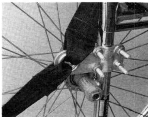
Fig. 1. Safe-N-Sound wheelchair and occupant restraint systems attached to rear upright of wheelchair.
