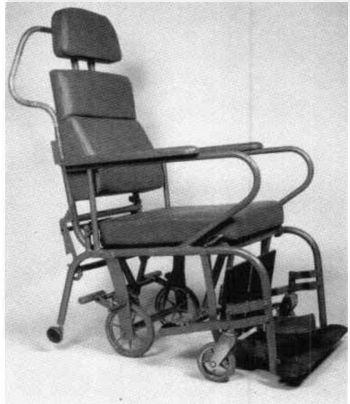
Fig. 8. A chair with wheels just behind the centre of gravity.
