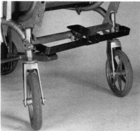
Fig. 7. Improved braking system.
