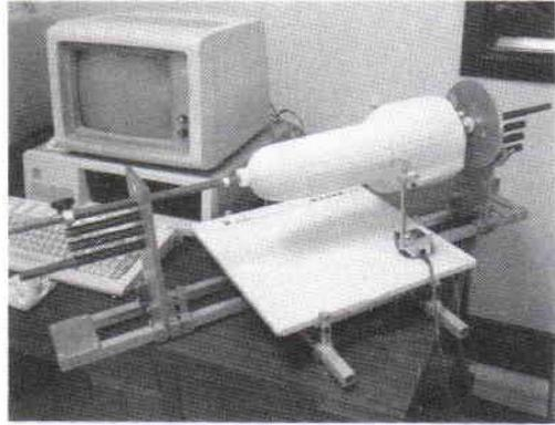
Fig. 2. Shape Copier device used in the digitization of the reference shape positive casts.
