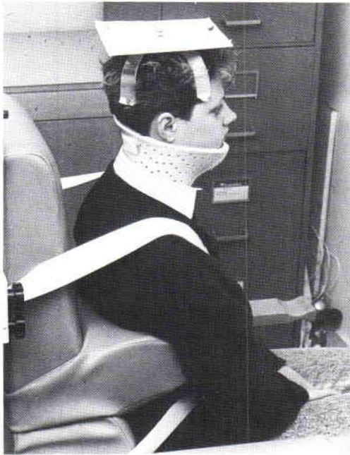
Fig. 2. Subject seated in test position for head rotation measurement using a horizontal goniometer.
