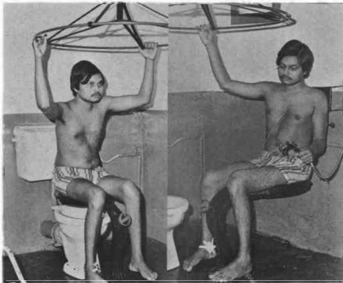
Fig. 1. Left, "Lawry" rotary attachment. Transfer is facilitated by use of the overhead support. Right, the rotary attachment is swung away from the water closet seat for washing. Note the water tap just below the back rest and separate shower hose.
