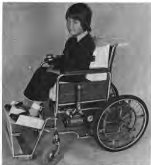
Fig. 9. Completed modular seat for a patient with muscular dystrophy.
