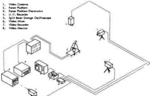
Fig. 5. Schematic diagram of gait analysis apparatus.
