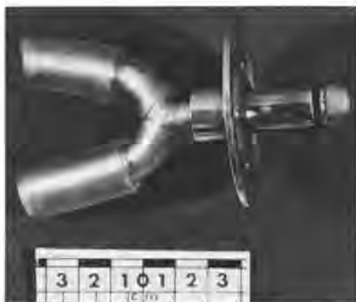
Fig. 1 The fixed-hook driving appliance. The forks of the 'V' are covered by rubber tubing.
