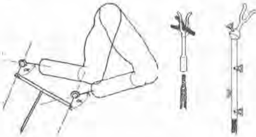
Fig. 2 Left, the use of the ball-and-cup driving appliance. The angle \alpha changes depending upon the position of the wheel. Right, gear lever attachments for use with the driving hook. The simple attachment is shown on the left, the adjustable appliance on the right (see text).
