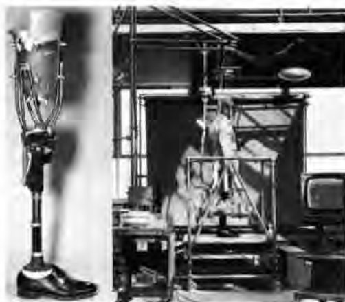
Fig. 5. Left, trial prosthesis showing adjustable socket mounting, transparent socket and built-in transducers. Right, subject on experimental rig, note overhead hoist and harness with weights attached.
