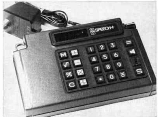
Fig. 6. Talking output calculator for the blind.
