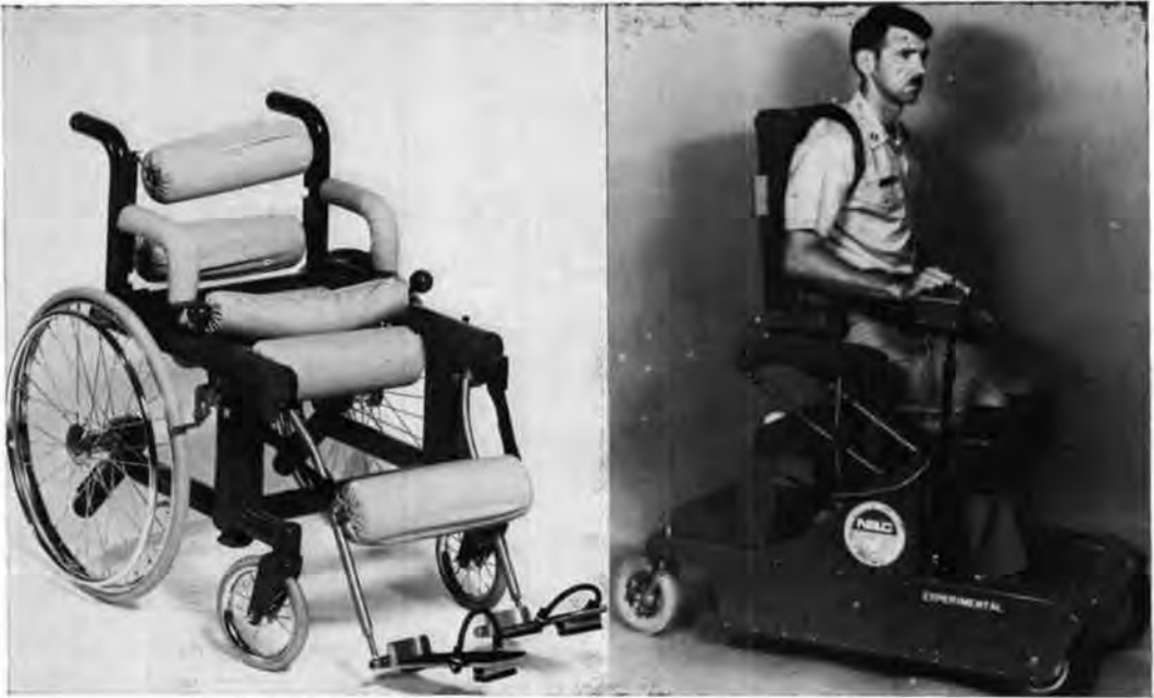
Fig. 2. Left, stand-up wheelchair. Right, powered stand-up mobility system.
