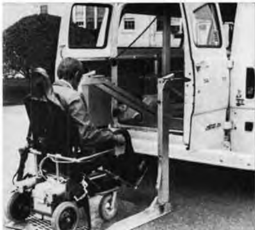
Fig. 4. Automatic wheelchair lift system for a passenger vehicle.
