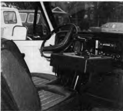
Fig. 3. Adaptation of the joystick controlled vehicle used on the moon.
