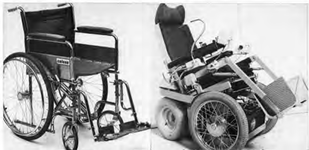
Fig. 1. Left, typical manually propelled wheelchair. Right, an example of a heavy, multi-purpose wheelchair.
