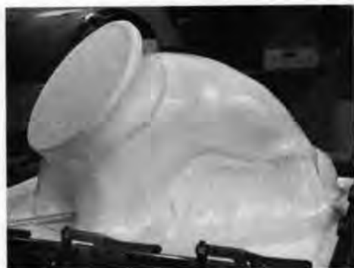
Fig. 3. A second layer of ABS is vacuum formed to locate the base plate and stiffen the seat.
