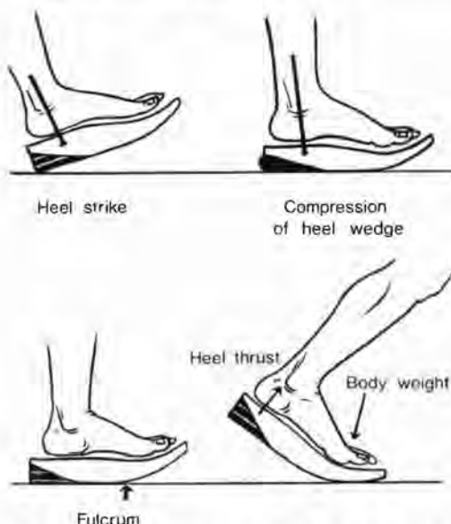
Fig. 12. With the foregoing design, an ankle joint is not needed. The orthosis can be quickly and very economically fabricated.
