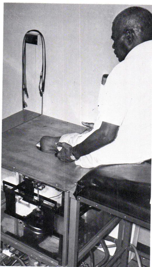
Figure 1-A. A patient's residual limb is scanned by the ultrasound shape sensing device.
