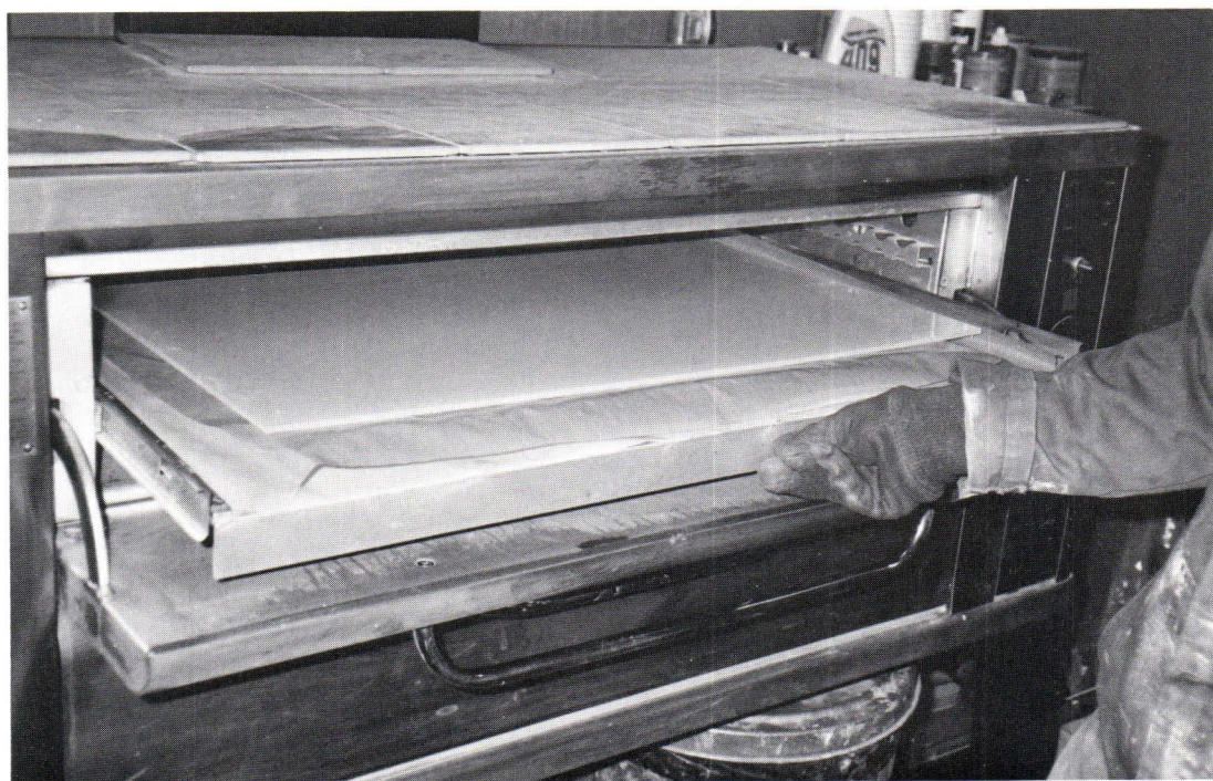
Figure 4. The "sandwiched" plastic sheets are placed in the oven together.
