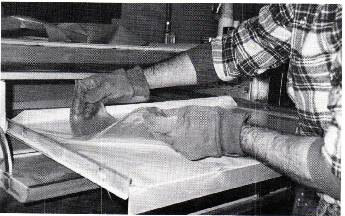
Figure 6. The second sheet of plastic is now ready to apply to the positive model.
