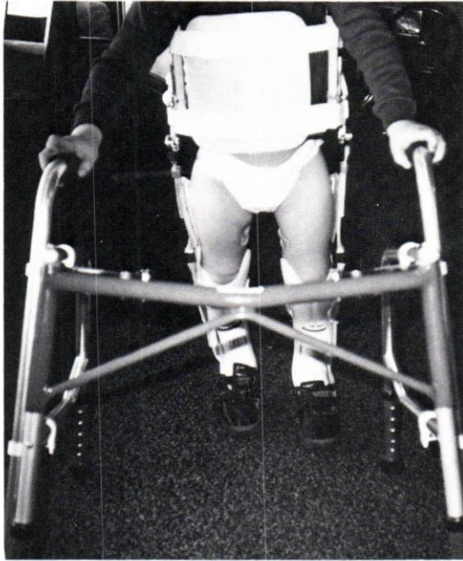
Figure 1. Reciprocating Gait Orthosis utilizing single lateral uprights and polypropylene pretibial shells.
