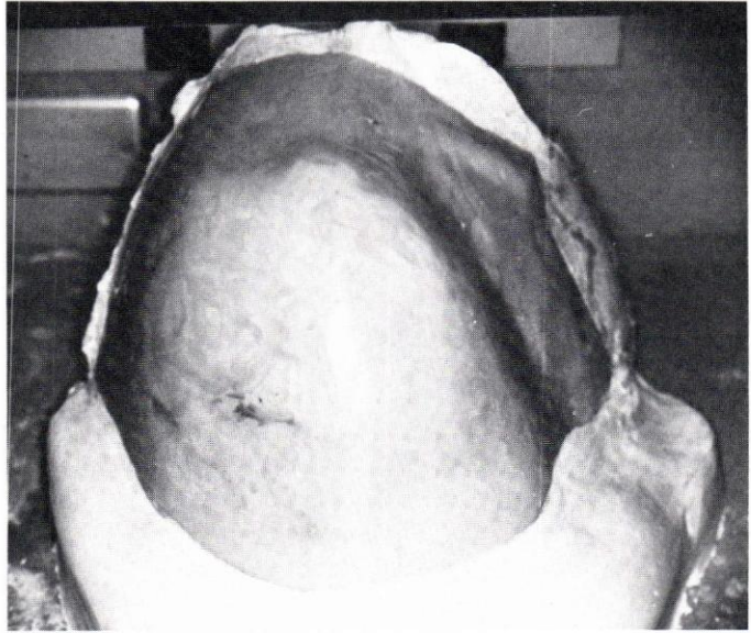
Figure 5. (left) Top and bottom of the mold are separated after the wax is boiled off, prior to tin foil substitute preparation.
