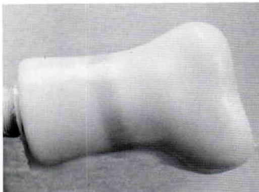
Figure 3. Vacuum formed colyene over positive model.
