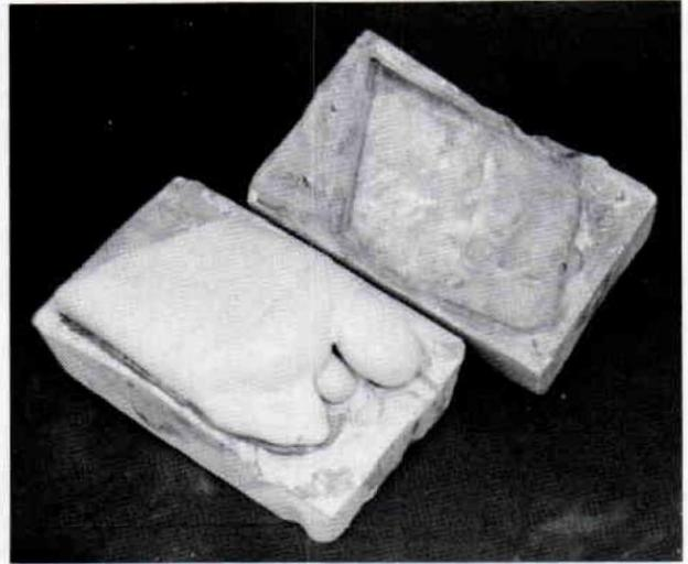
Figure 5. Mold halves with positive model.
