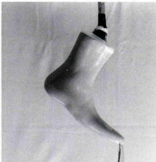
Figure 7. Lamination with rubber epoxy resin (Lynadure®).
