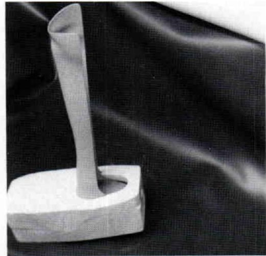
Figure 10. Flexion alignment of socket in mold.
