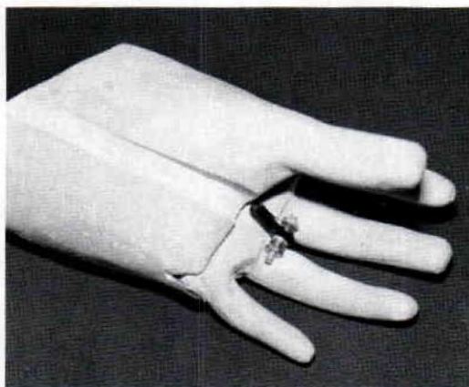
Figure 18. The pivot joint is prepared for attachment to the finger unit.
