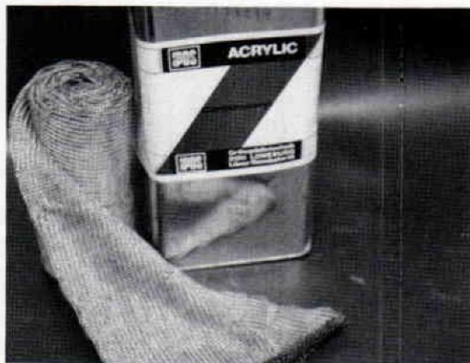
Figure 1. I.P.O.S. Carbonacryl ® resin and carbon fiber and fiberglass stockinette.
