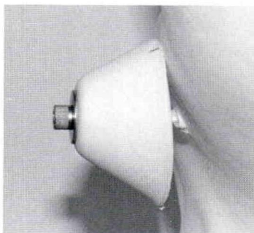
Figure 4. Lug mount assembly and alignment rod inserted in hole in model.
