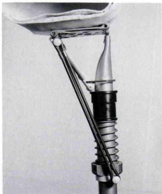
Figure 5. Otto Bock 7E4 hip joint with hip flexion bias system (HFB) added for initiating hip flexion.
