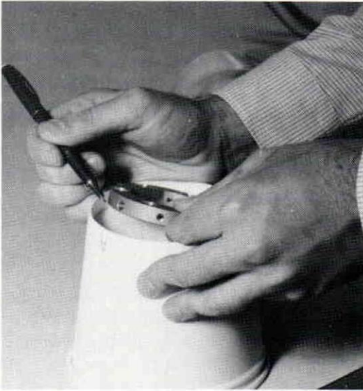
Figure 3. The top ring from the adjustable leg is aligned to the cup and its hole pattern is marked.
