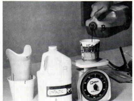
Figure 8. Syntactic resin is mixed in a 50/50 ratio by weight.
