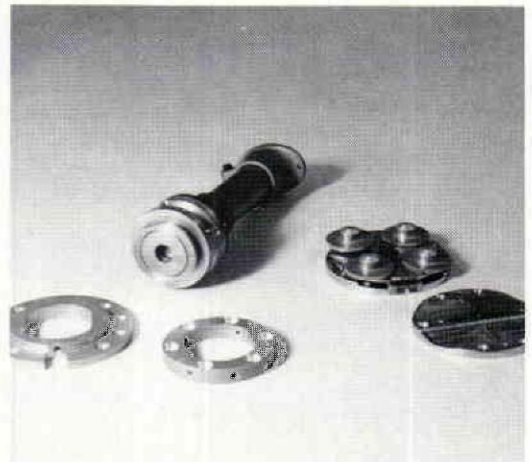
Figure 2. Hole patterns in alignment couplings vary greatly.
