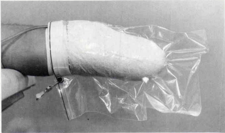
Figure 14. Apply vacuum (20 to 30 inches of mercury).
