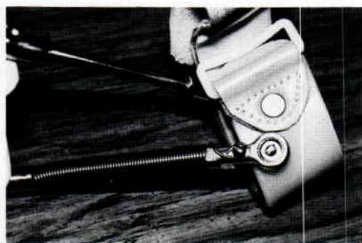
Fig. 7. Distal rod end bearing attached to polypropylene wrist cuff.
