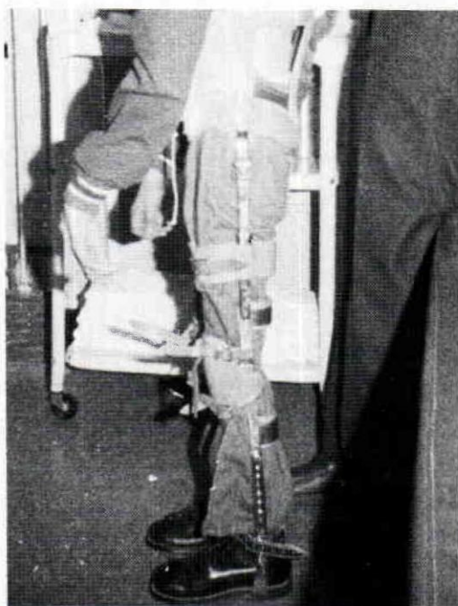
Fig. 3. Conventional double upright designs are bulkier and have a higher incidence of breakage.
