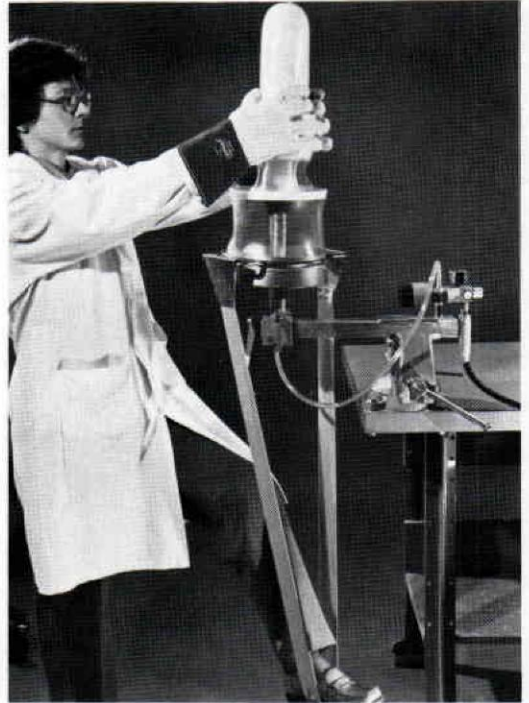
Fig. 3. Vacuum forming a transparent test socket.
