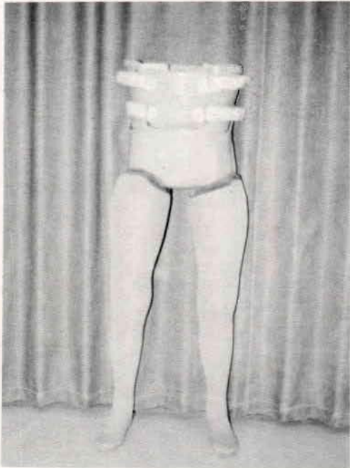
Fig. 10—The socket keyed into the prosthesis in a standing position.
