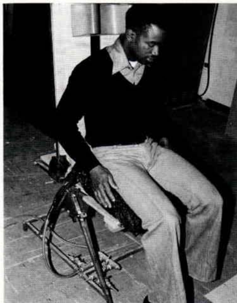
Fig. 3—The dilatancy bag is smoothed and placed on the seat. After the seat depth and angle has been set, the patient sits on the bag and is comfortably positioned. Vacuum is applied and the cushion becomes firm, leaving a negative impression. Partial vacuum may be used to modify the impression.
