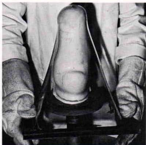
Fig. 6. Vacuum forming a transparent socket for a below-knee prosthesis.
