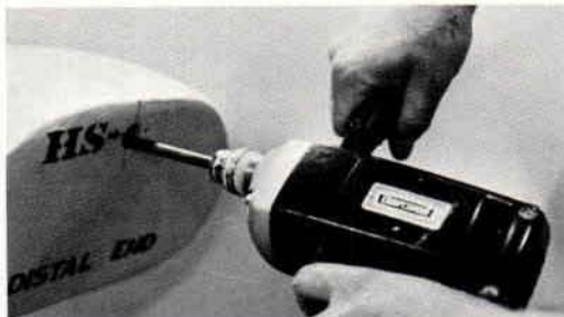
Fig. 3. The drill bit must be held level to posterior surface. It must not deviate from mid-line when drilling shaft. H.S. — horizontal shaft.
