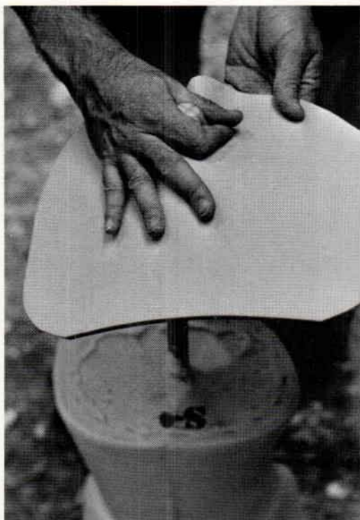
Fig. 12. The polyethylene foam Plastizote end cap is heated and a nipple is formed to be used to secure end cap to pipe.
