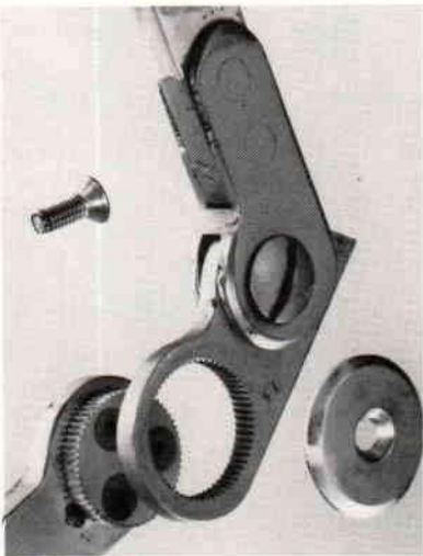
Fig. 20. The Dial Knee Unit disassembled.
