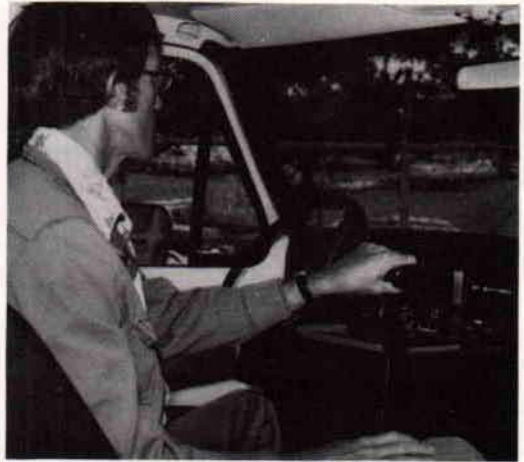
Fig. 9. Another form of joy-stick control: — an adaptation of the lunar rover module control developed by NASA for the Apollo project.
