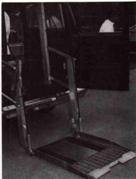
Fig. 7. A lift system for wheelchair access to a vehicle. This kind of item requires professional engineering inspections at installation and periodically thereafter.
