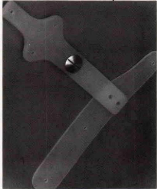
Fig. 1. The polypropylene pelvic joint and band, assembled.
