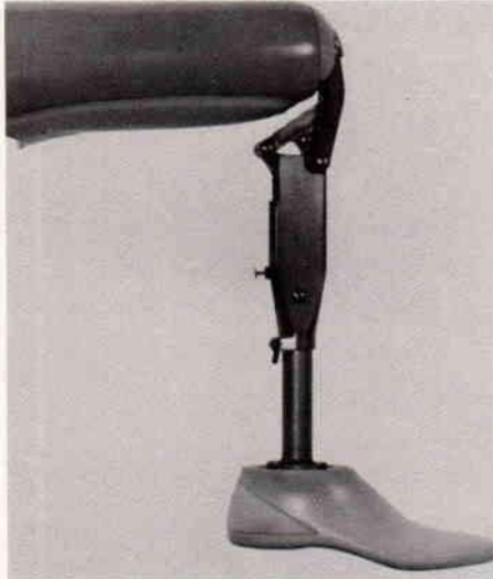
Fig. 2. The OHC knee-disarticulation prosthesis in flexion. Flexion is limited to about 100 deg. but this seldom presents a problem to most lower-limb amputees.
