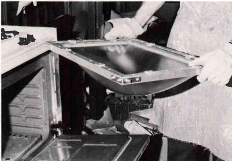
Fig. 3. The molten plastic sheet being removed from the oven prior to placement over the male model. Note the special frame, or rack, for holding the plastic sheet around the periphery.
