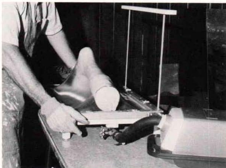
Fig. 5. The plastic sheet and frame are brought in contact with the vacuum table so as to seal the enclosed area with respect to the atmosphere.
