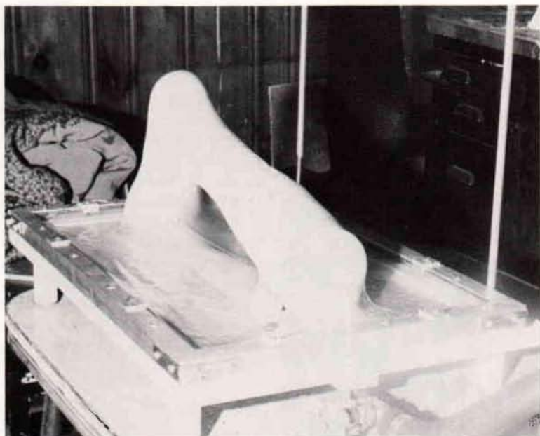
Fig. 6. The air underneath the plastic is pumped out and the plastic follows the form made by the model and table. The form is retained faithfully by most sheet plastics upon cooling.
