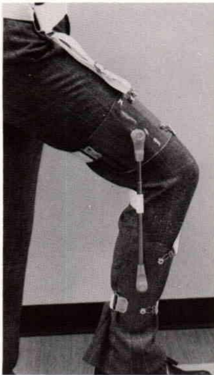
Fig. 4. Lateral view of experimental orthosis to show action of the telescoping assembly.
