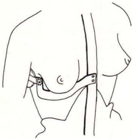
Fig. 2. New L-bracket for the Milwaukee orthosis.
