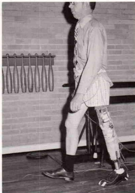
Fig. 2. Above-knee amputee subject walking while using instrumented prosthesis to record gait characteristics.
