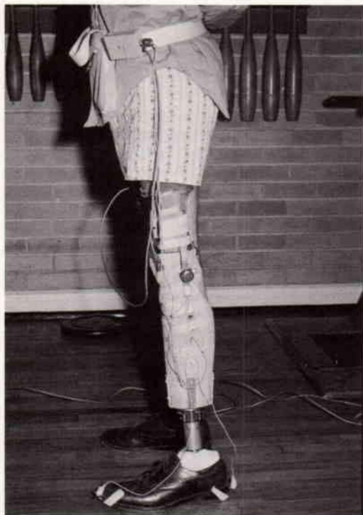
Fig. 1. Instrumented prosthesis for measuring characteristics of gait of above-knee amputees.
