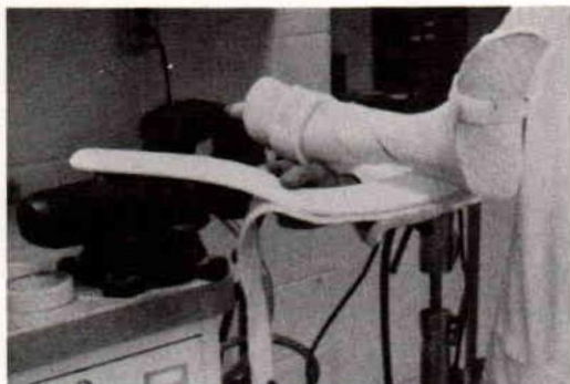
Fig. 2. Application of felt patterns needed to apply uniform loading over the softened polypropylene.
