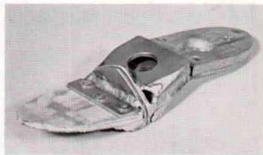
Fig. 2. Special keel assembly for use in construction of a molded SACH foot.
