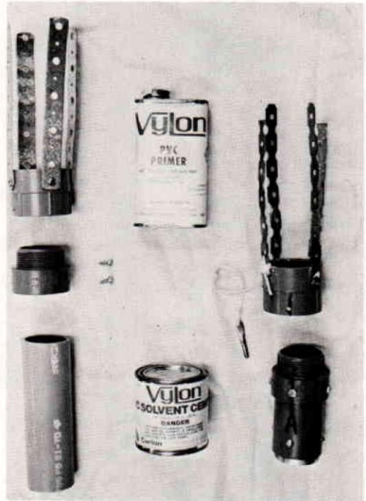
Fig. 1. Various components of the plastic pylon. The primer and solvent cement are shown also.
