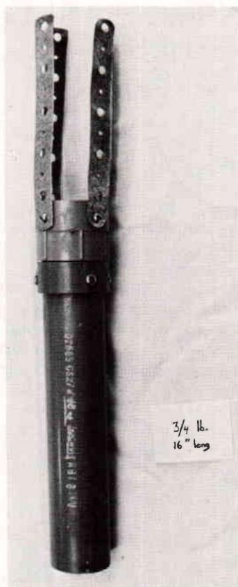
Fig. 2. An assembled pylon with galvanized straps.
