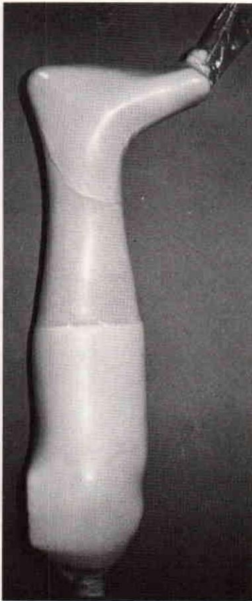
Fig. 24. The prepared positive mold, covered by a second PVA foil, is ready for lamination.
