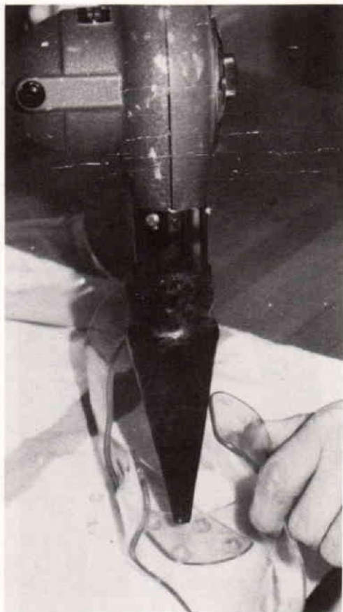
Fig. 12. Heating the shrink-expansion rivets with heat gun with funnel attachment.
